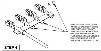
**NOTE**: COMMERCIAL CRIMPERS FOR "B" CRIMPING ARE VERY COMMON AND SHOULD BE USED ON SINGLE TERMINALS. HOWEVER, THEY DO NOT FULLY MEET FACTORY CRIMP SPECIFICATIONS SO SOLDERING IS RECOMMENDED.
