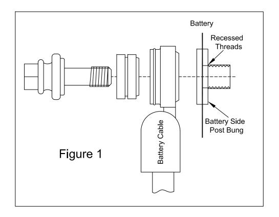
Many new side post batteries feature recessed threads on their side post bungs (See Figure 1). This often causes problems with the older short cable attachment bolts (See Figure 2). The bolt must engage the battery bung threads for at least 3-1/2 threads for a proper secure connection.
