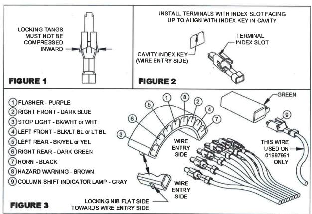
For ease of installation, we have left the plastic connector off of the end of the turn signal switch.
