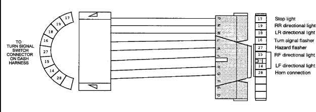
LR directional light TO TURN SIGNAL SWITCH CONNECTOR Turn signal flasher
